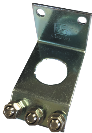
GP 003/20 - manufactured from 2mm thick brass with 2 x 5mm fixing holes, supplied with brass earthing stud, nut and washer.
